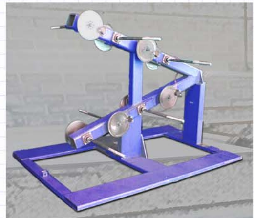
ILLUSTRATES MODEL 438-1B EIGHT REEL DE- REELING AND TENSION STAND
