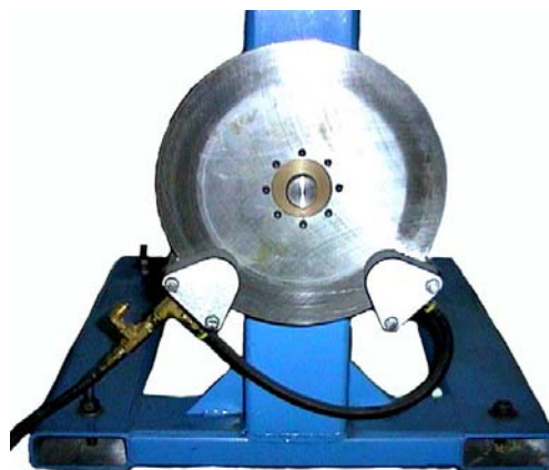
ILLUSTRATES MODEL 432-2B DOUBLE BRAKE FOR ADDITIONAL TENSION
