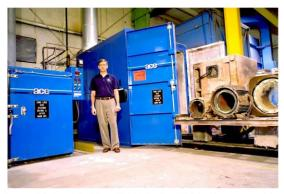
Mr. Dan Parsons (EASA Travelling Chiefs) of AC Electric, Bangor, ME stands in front of the two ACE Burn Off Ovens at the facility. The oven to the left is the -RKG- model. The oven to the right is the new HYBRID Radiant Tube Oven system.
