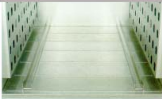
Insulated Floor with Surface Truck Tracks used where oven will be recessed into the factory floor or loaded with an external ramp, includes drag seals on the oven doors. Total track loading limited to distributed floor loading of 100 lbs per square foot.
