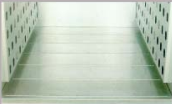
Insulated floor with steel plate cover, 2" for 500°F and 650°, 3" at 750°F, minimizes heat loss and improves temperature uniformity near floor level, rated at 100 lbs per square foot distributed
