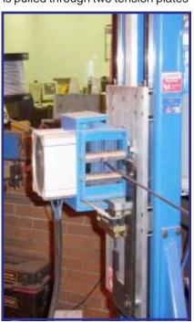
the Tension Device), thus creating Force (F) on the Tension Sensor. The **Tension Sensor** measures the amount of Force (F) and transmits an input signal to the Tension Controller. The Tension Controller compares the tension of Force (F) against the setpoint and reduces the signal deviation to zero by increasing or decreasing the output signal to the Converter.
