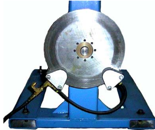
ILLUSTRATES MODEL 432-2B DOUBLE BRAKE FOR ADDITIONAL TENSION
