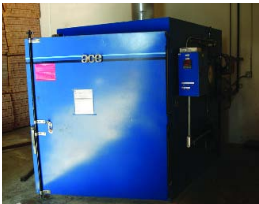
Hannibal Industries uses this burn-off oven to remove powder buildup from its hangers.
