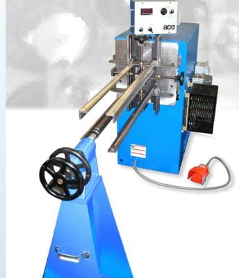
A 1.25" square center support post is mounted in the center of the main support base and extends the full length of the form. The four corner angle bars are supported on the end and middle by adjustable support plates extending from the square center post. These supports provide rigidity and the four corner angle bars from collapsing inward during winding.
