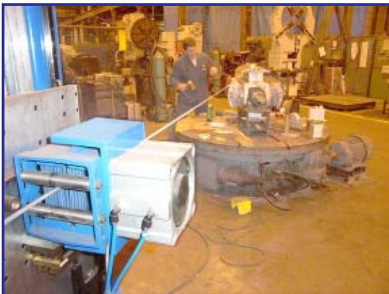
The Model 4810V-TC82 provides proper tension when winding specialized rotors resulting in a tight coil for a perfect fit. There is no damage to the wire or equipment and minimal operator manipulation is required.
